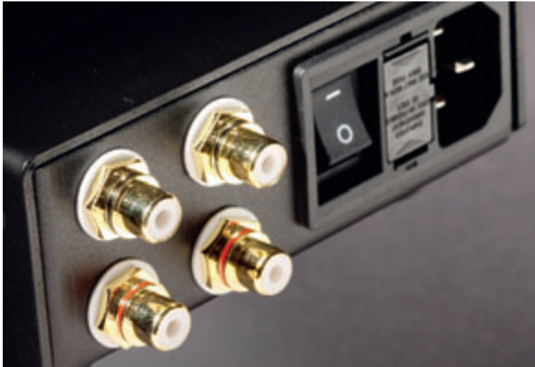
ABOVE: Not two inputs but a combination of L/R stereo input and variable preamp output, controlled off the same volume control as the two front headphone sockets
