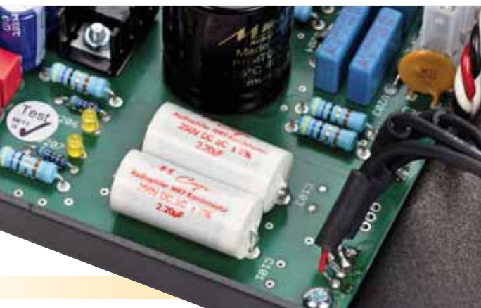
Among the high-grade components on the pc board there are also several capacitors from the Cologne-based specialist Mundorf
