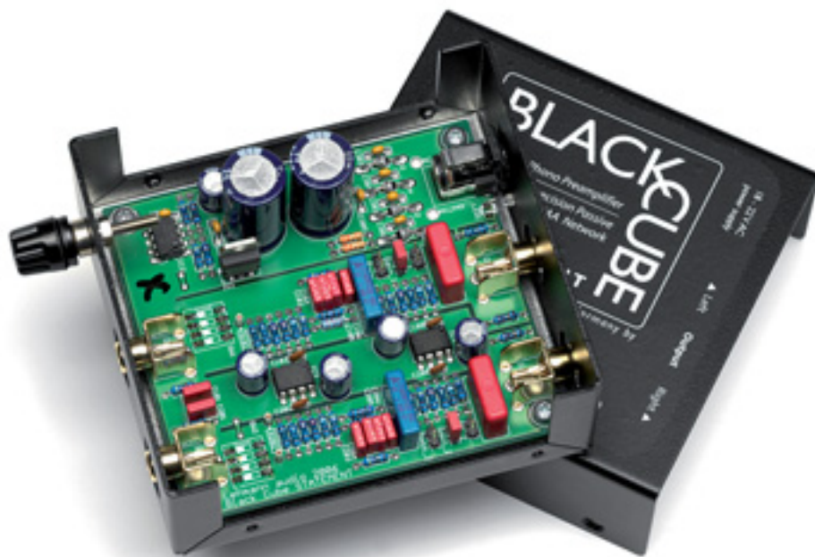
Sensibly high-quality components in a compact design. Not pictured: the power supply.
